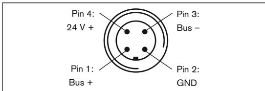
Bus connection with external supply voltage (optional)
