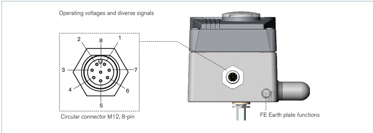
**Circular connector M12 - 8-pin (Input signal)**
