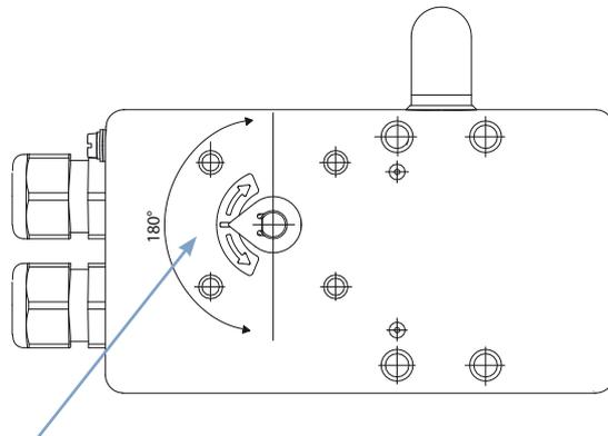
The rotation angle of the sensor must be within a range of 180°
